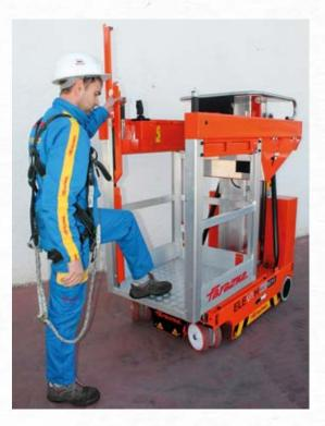
Automatic cage locking. Anti-tilting device. Electronic slope monitoring. Electronic braking system. Overload monitoring Emergency hydraulic lowering.
