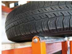
**OPTIONAL:** possibility of adding an arm with lifting ropes for stowing tyres flat. It helps to move the tyres from the tool to the shelf without lifting it. The operator doesn't make any effort and always keeps the correct position
